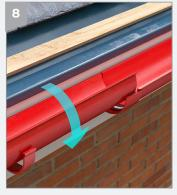
Repeat step 5, then firmly place the male end of the gutter or accessory onto the siliconed strap joint. Ensure the top of the gutters are fully aligned.
