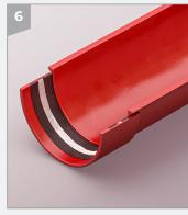
Prior to assembling gutter joints ensure that all fixing surfaces are clean and dry. Apply 2 strips of butyl tape (GM32) 10mm apart inside the joint strap of the gutter. Fill the 10mm gap generously with silicone sealant (GM30), do not remove any excess.
