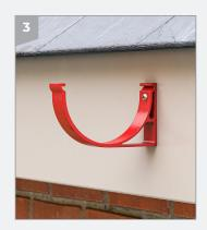
Fix a fascia bracket at each end of the run with a 38 x 5 stainless steel screw (GM1).
