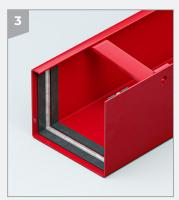
Prior to assembling gutter joins ensure that all fixing surfaces are clean and dry. Apply 2 strips of butyl tape (GM32) 10mm apart inside the female end of the gutter. Fill the 10mm gap generously with silicone sealant (GM30). Do not remove any excess.
