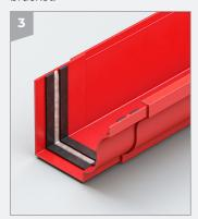
Prior to assembling gutter joints ensure that all fixing surfaces are clean and dry. Apply 2 strips of butyl tape (GM32) 10mm apart inside the female end of the gutter. Fill the 10mm gap generously with silicone sealant (GM30). Do not remove any excess.
