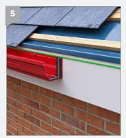
Using a string line or laser level mark the position of the remaining gutter lengths.
