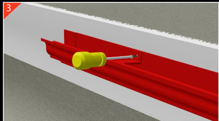
Once the position is established the first length can be fixed (level), directly through the cross-brace in the back of the gutter using 38 x 5 stainless steel screws (Guttercrest GM1).
