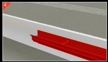
Next use a string / laser line, to determine the position of the remaining gutter lengths in the run. We recommend a level fall, If a fall is required - max. 1:600.
