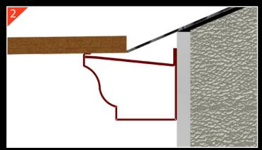
Alternatively use a spirit level against the lowest point of the roof tile to determine the position the gutter is fixed .\*
