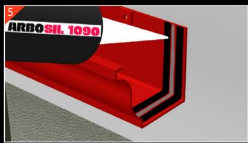
To join the next length of guttering, lay 2 strips of butyl tape (GM32) 10mm apart, inside the female end of the gutter, the tape is manually bedded into the corners of the gutter profile. The 10mm gap is then liberally gun filled with the recommended silicone sealant (GM30). The silicone is left proud with no excess removed.
