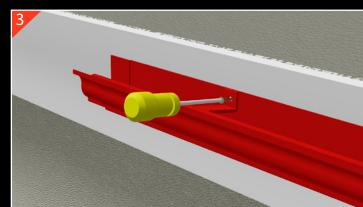
Once the position is established the first length can be fixed (level), directly through the cross-brace in the back of the gutter using 38 x 5 stainless steel screws (Guttercrest GM1).
