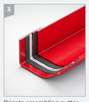
Prior to assembling gutter joins ensure that all fixing surfaces are clean and dry. Apply 2 strips of butyl tape (GM32) 10mm apart inside the female end of the gutter. Fill the 10mm gap generously with silicone sealant (GM30). Do not remove any excess.
