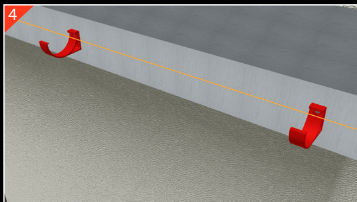
Repeat the above steps at the other end of the gutter run. Then use a string / laser line between the two ends and continue to fix the fascia brackets at 900mm centers. We recommend a level fall, if a fall is required - max. 1 : 600.
