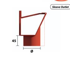
\* Indicates a sleeve outlet can be used in place of running outlets giving increased flexibility and cost efficiency.
