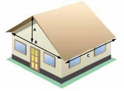
Effective roof area =  $(A/2 + B) \times C = ERA M$ RUN OFF Run off = effective roof area x rainfall intensity = I/s
